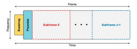
Figure 7.10 from "A/322: ATSC Candidate Standard – Physical Layer Protocol" shows the frame structure of an ATSC 3.0 frame. The bootstrap at the start of the frame provides the information necessary to demodulate the preamble, which in turn provides the information necessary to demodulate the rest of the data in the frame and its subframes.
